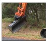
Wedgelock I-Lock<sup>™</sup> Tilt Coupler A high level of Safety - the I-Lock Tilt<sup>™</sup> Coupler provides a guaranteed instant, independent and innovative safety system in a tilt-coupler. The unique Elliptic Rotary Actuator delivering up to 60% more digging force at the bucket tip.
