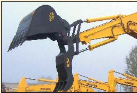
SERIES II PROFILE FOR PIN GRABBER Q.C. UTILIZE THUMB WITH MULTIPLE ATTACHMENTS
