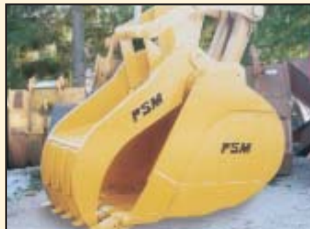
LOG PROFILE AGGRESSIVE RADIUS CRADLES ROCK, LOG, DEMOLITION DEBRIS
